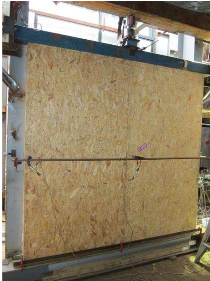
Figure 15: Axial load test setup
