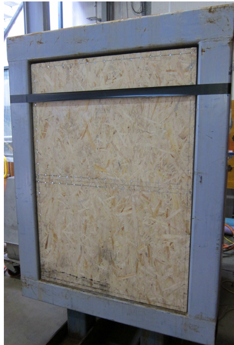
Figure 17: Test specimen during Low-High-Low fatigue testing
