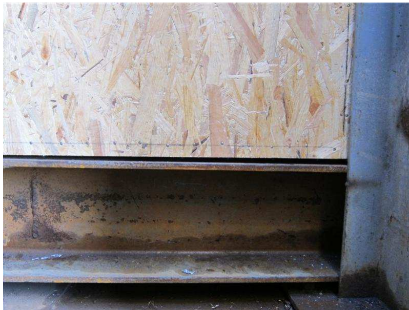
Figure 13: Specimen lifting off the test rig during racking test because of fixings pulling through the timber base plate
