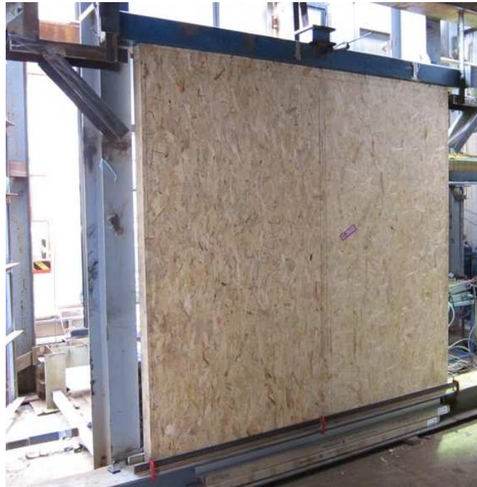
Figure 12: Test specimen installed in racking resistance and axial loading rig
