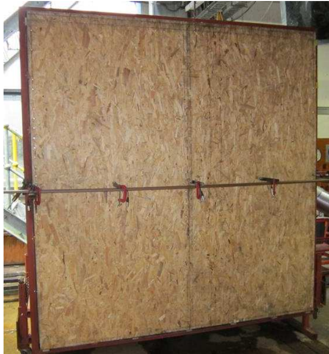
Figure 16: Wind load resistance test setup in pressure rig, transducers mounted along horizontal
