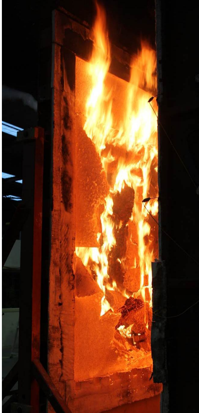
Figure A6.4 Exposed face of specimen at the end of the test
