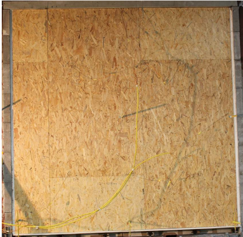
Figure A6.1. Unexposed face of specimen before commencement of the fire-resistance test.
