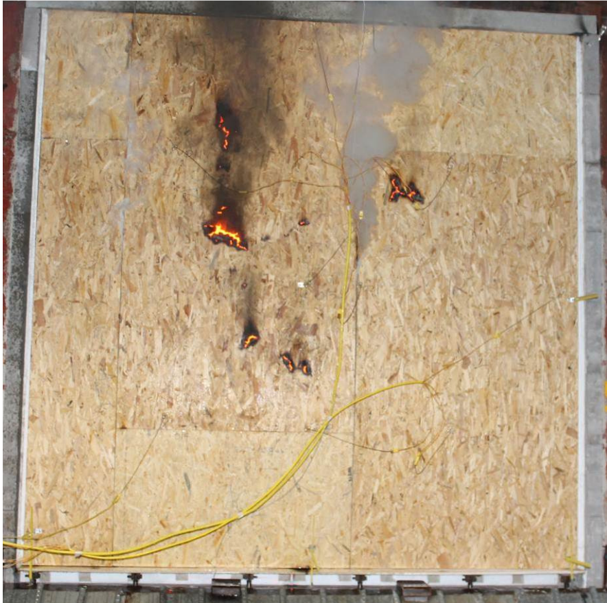
Figure A6.3. Unexposed face of specimen at the end of the test
